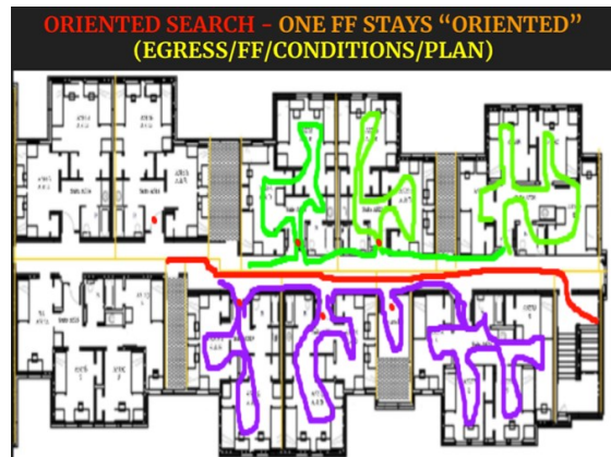
The diagram shows a public hallway apartment building with a three firefighter crew. The red represents the "oriented" firefighter, while the green is firefighter one and the purple is firefighter two which are searching simultaneously.
